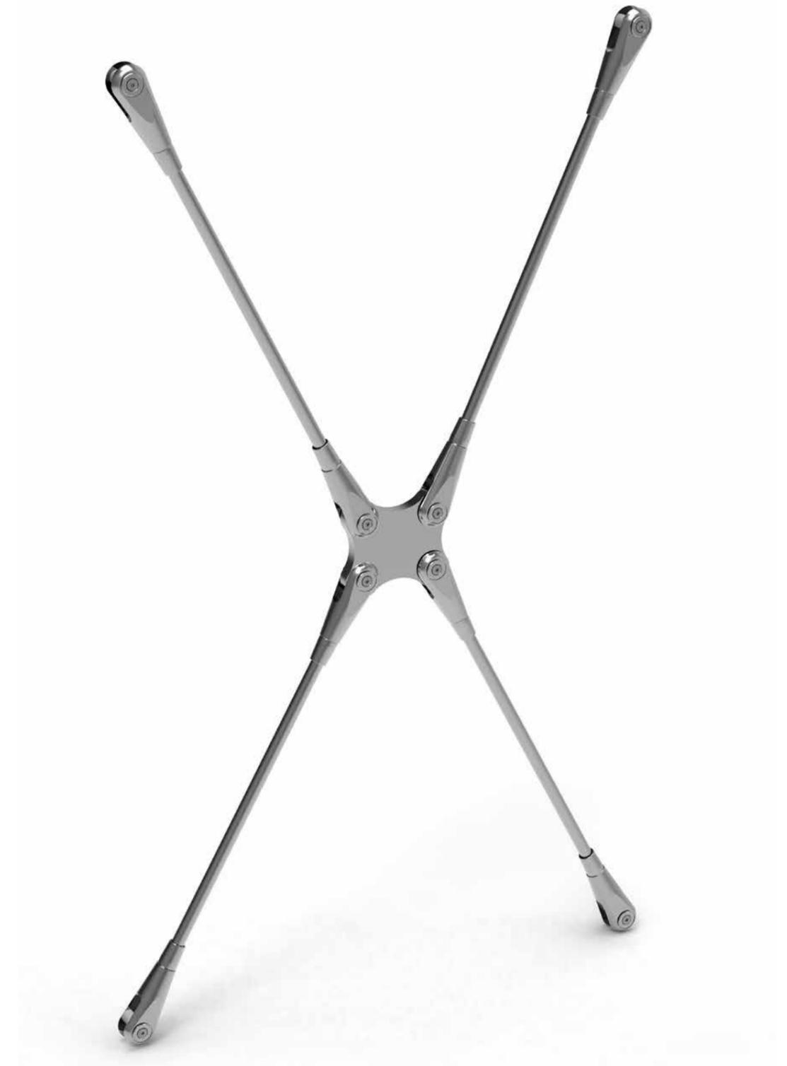
Rod systems are used in many fields of applications such as canopies, bracing of glass façades, bridge constructions and pedestrian bridges, as well as bus stations and airport buildings. INOX-NET I-ROD systems are suited for a wide range of applications from M10 up to M30 sizes with individual rod lengths up to 6m. All systems are delivered pre-assembled and ready for installation.
